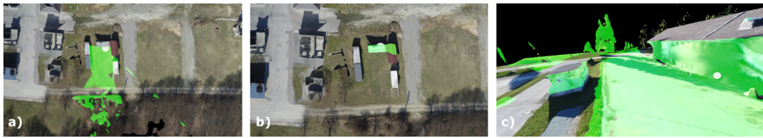
Figure 5.4: The visibility tool helps to analyze line-of-sight from a chosen position. a) The sphere is placed in the corner of a building. Visible areas from the position of the sphere are colored in a green shade. b) If the sphere is placed inside a building, nothing outside the building is visible. Image c) shows that from the current position of the sphere, people would not see the bottom of the house on the left side.
