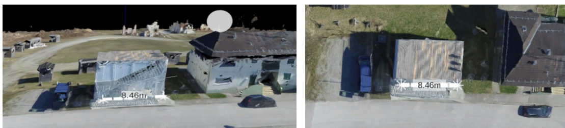
Figure 4.19: A measurement object indicating the distance between two points in 3D. A measurement object is shown Left: from the perspective of the immersed user and Right: from the perspective of the desktop user.
