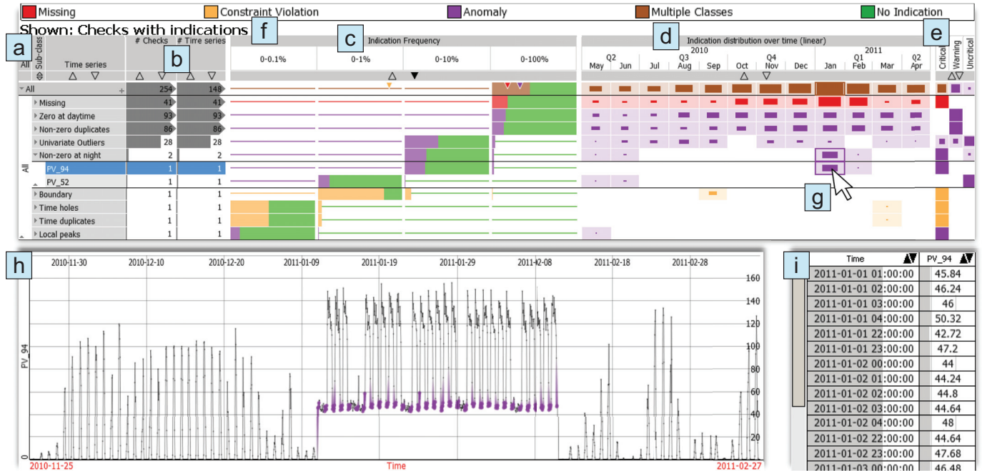
Fig. 2. Visplause consists of multiple linked parts. The DQ overview provides a hierarchical overview of check results (a). In this example, checks are aggregated by ‘Sub-class’ and ‘Time Series’ to reveal the most prevalent types of DQ issues and their source. DQ overview columns show additional information such as (b) the number of checks and time series, (c) the percentage of affected data, (d) the distribution of check indications over time and (e) the severity of check indications. (f) The current filter shows only checks with at least one check indication. (g) Non-zero at night anomalies at power plant PV_94 in January 2011 have been selected. (h, i) Linked views provide details of the selected data anomalies for validation.
