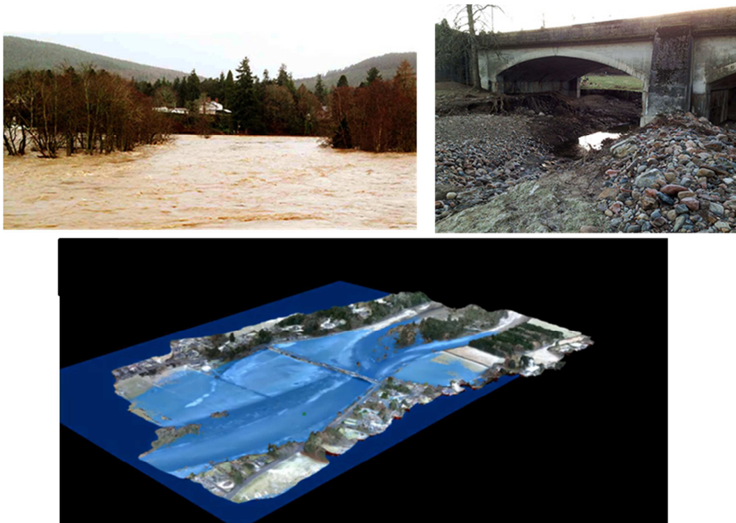
Figure 2: Flooding in Aboyne. Images such as the upper left can be used to recreate a hydrograph by superimposing flood levels on the DEM (lower). The results can be used to model the impact of flood related scour under the bridge (upper-right).
