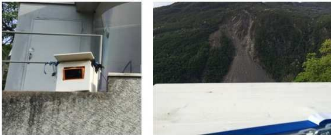
Figure 1: Field setup of the real time TLS monitoring system using Optech Ilris LR scanner.
