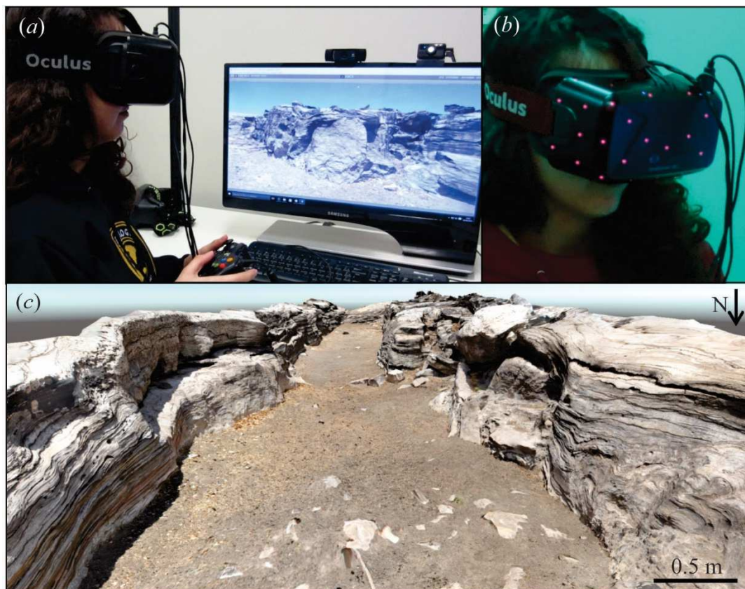
Figure 1: The system prototype, highlighting a) user interacting with the application through head-mounted display and game controller; b) infrared view of the Head Mounted Display, where red points are part of the HMD tracking system; c) virtual 3D outcrop model, obtained by multiple images and SfM techniques.
