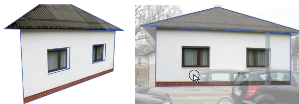
Figure 5: Left: By defining hierarchical relations, holes and side faces are automatically extracted. Right: Interactive removal of occluding objects from the texture by overlaying the photo semi-transparently using the Shot view.
