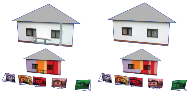
Figure 6: Top left: The initial texture containing occluders. Bottom Left: The associated Shots, visualized using a false color mask. Top right: The cleaned texture after interactive brushing. Bottom right: The correspondingly modified mask.
