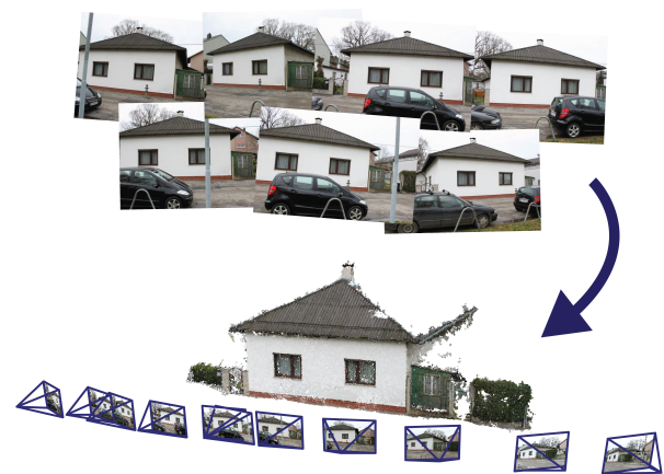
Figure 2: Photogrammetric Network (bottom), consisting of a 3D point cloud and photos (top), for which their relative positions and orientations have been computed. We refer to them as Shots in this work.
