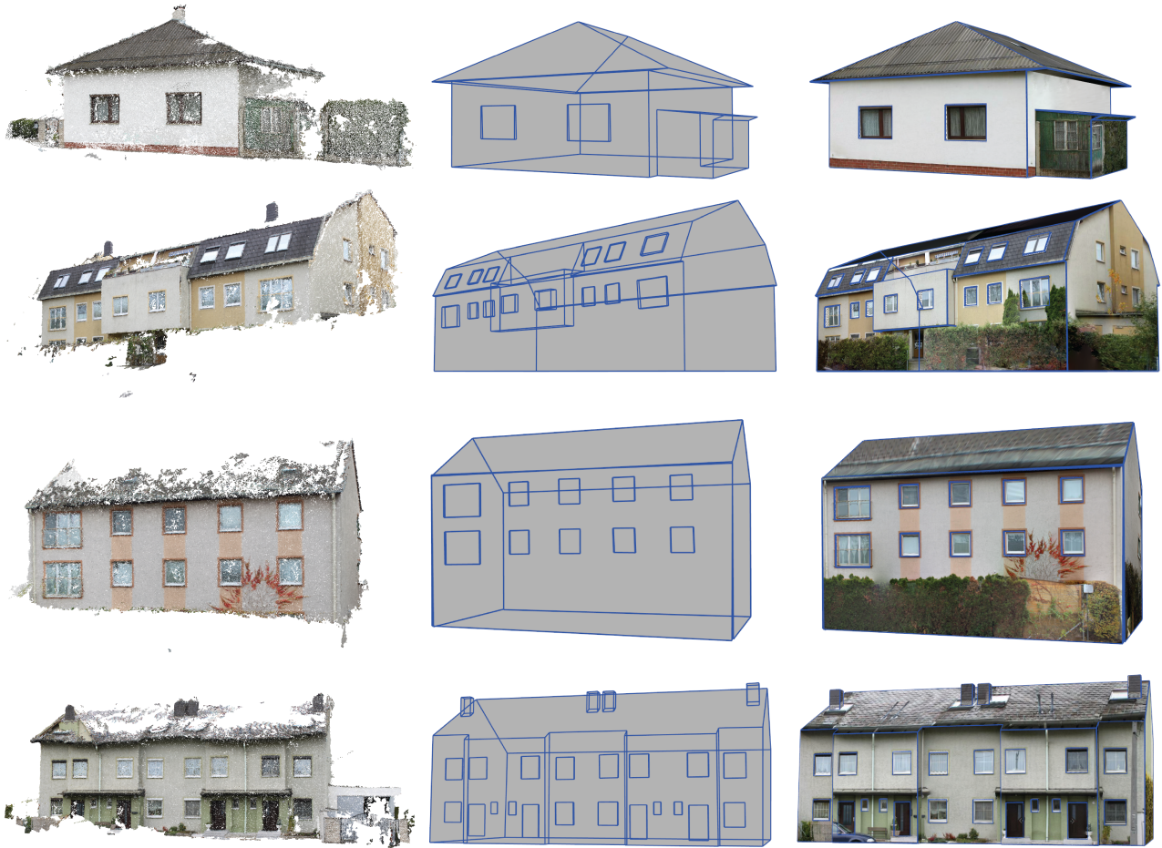
Figure 7: Three textured 3D building models generated with our approach. In the left column, the photogrammetric point cloud is visualized, followed by the geometric reconstruction including hierarchical definitions in the middle column. In the right column, the final model with textures generated from multiple photos and using interactive occluder removal are shown. While parts that are not depicted in the point cloud could be reconstructed using the photos, that the backsides of the houses were modeled freely, as they were not accessible for the photographer. Modeling time including texture generation: Top row 5 minutes, seconds row 15 minutes, third row 10 minutes, fourth row 20 min.
