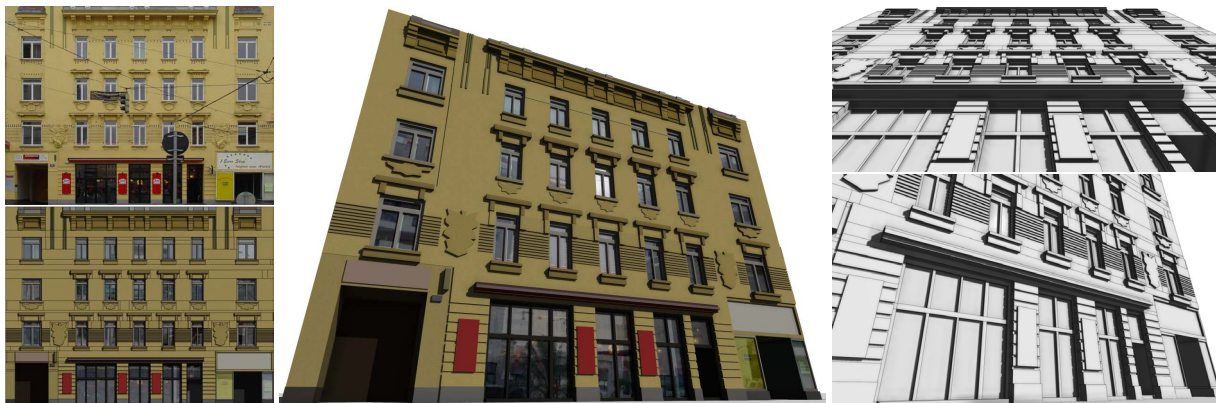
Figure 1: Starting from an orthogonal input image (left top), the user interactively segments the façade into shapes (bottom left). Most split lines and symmetries are found automatically by the system, while the global façade structure is determined by the user. The input resolution is 1024 \times 756 , the number of visible shapes is 1346, and the modeling time is about 8 minutes (with material and depth assignments about 15 minutes).
