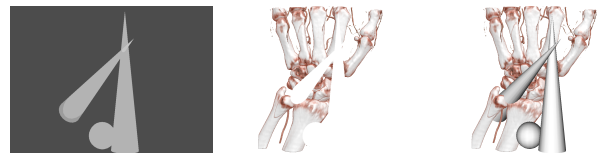
Figure 4: Intersections between volume data and OpenGL geometry exploiting the depth image of the geometry (left). During rendering, rays are stopped at the depth of the corresponding intersection points (center). Blending the geometry image on top of the volume yields the final image including correct intersections (right).
